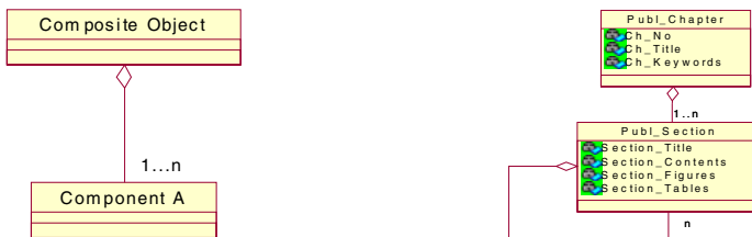
a. UML Notation for a Homogeneous Composition featuring One to Many relationship
