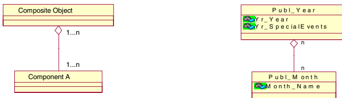
a. UML Notation for a Homogeneous Composition featuring Many to Many relationship
